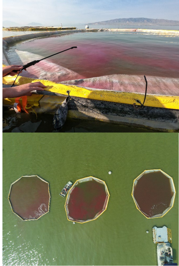
Figure 26 Dosing the corrals with rhodamine with the top panel showing the garden sprayer, and the bottom panel showing application to the middle corral.
