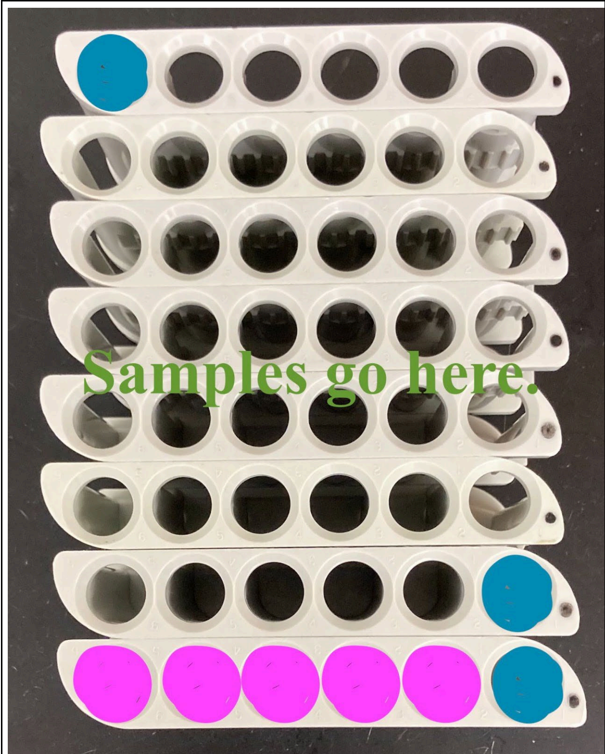
Milli-Q water spots are marked in blue, standard spots are marked in purple, sample spots are everywhere else. If you do not fill all eight rows, put the milli-Q vial in the spot after the last sample.
