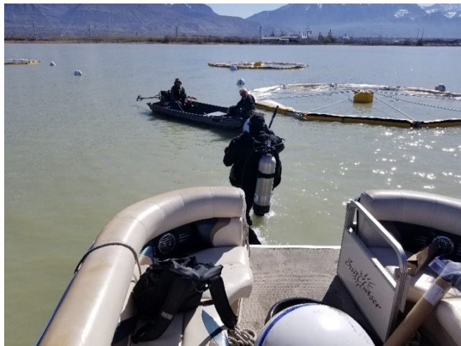
Figure 9 SCUBA diver and others working to anchor the corrals to the experimental site.
