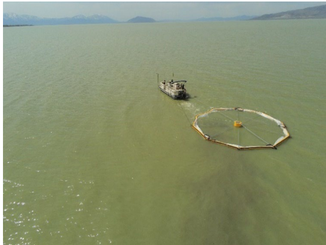
Figure 8 Towing the limnocorrals from the shore assembly site to the experimental site.
