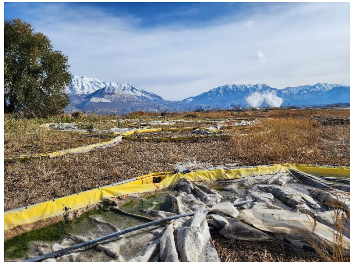
Figure 1 Limnocorrals on Shore showing the skirts
